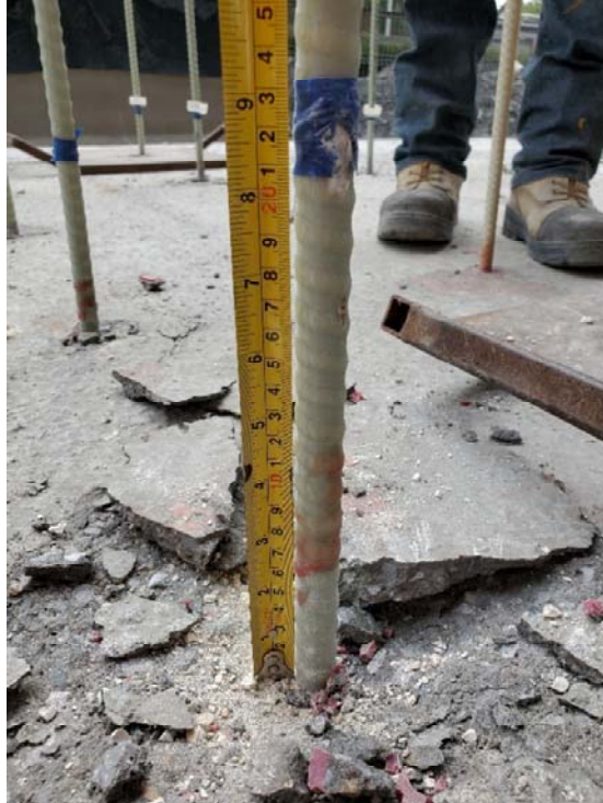
Figure 11 Pullout of GFRP from adhesive and concrete cone failure with the unconfined fibre-reinforced concrete (sample 3)
