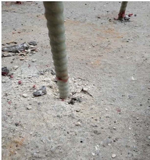
Figure 10 Pullout of GFRP from adhesive and concrete cone failure with the unconfined fibre-reinforced concrete (sample 2)
