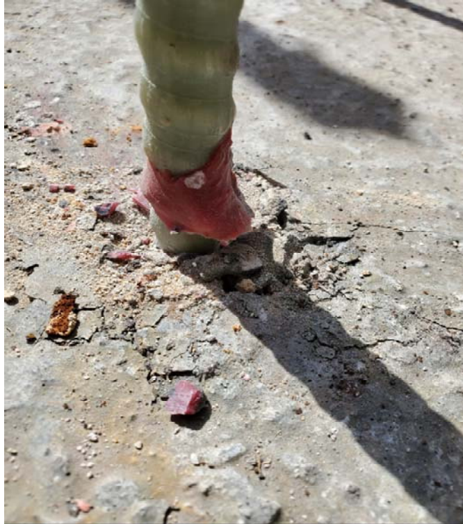
Figure 9 Pullout of GFRP from the adhesive in confined fibre-reinforced concrete (sample 5)
