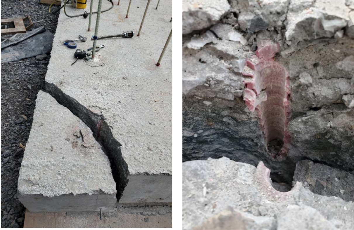
Figure 7 Shear failure in confined fibre-reinforced concrete (sample 2)
