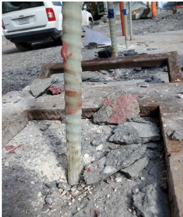
Figure 12 Concrete cone failure in unconfined fibre-reinforced concrete (sample 4)
