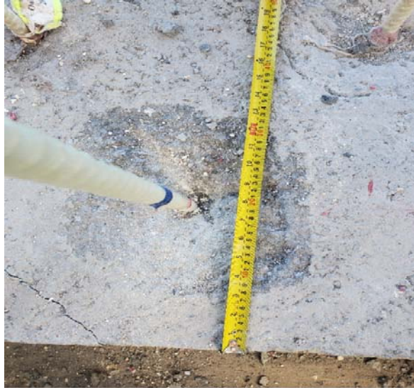
Figure 5 Pullout of GFRP from adhesive and concrete cone failure in unconfined normal concrete (sample 3)
