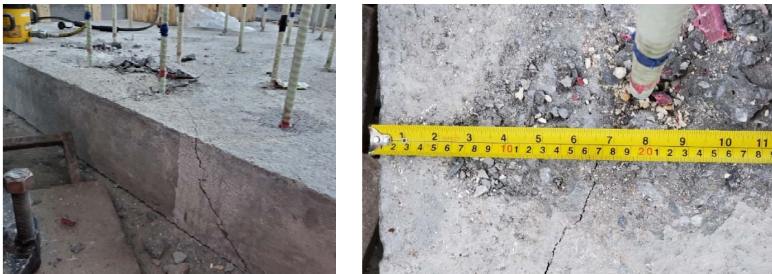
Figure 4 Example failure mode of slab shear failure (unconfined normal concrete sample 2)
