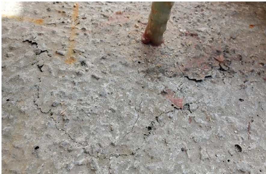
Figure 8 Test stopped before failure for H&S concerns in confined fibre-reinforced concrete (sample 3)
