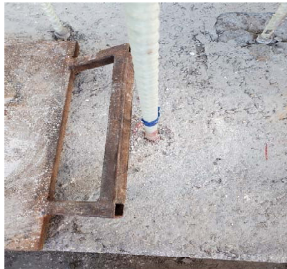
Figure 6 Pullout of GFRP from adhesive and concrete cone failure in unconfined normal concrete (sample 4)
